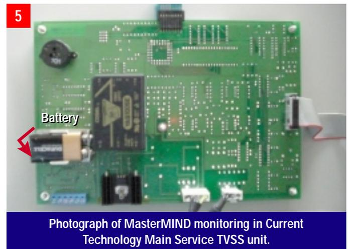
Photograph of MasterMIND monitoring in Current Technology Main Service TVSS unit.
