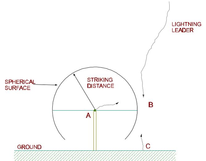
Figure 3 Spherical Surface with Striking Distance radius about point A
