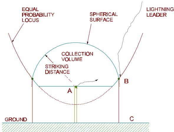
Figure 4. Collection Volume formed by equal-probability locus and spherical surface
